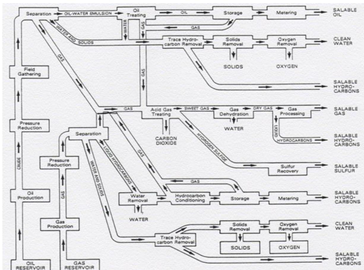
**Diagram #4: A simple example of oilfield flow**
